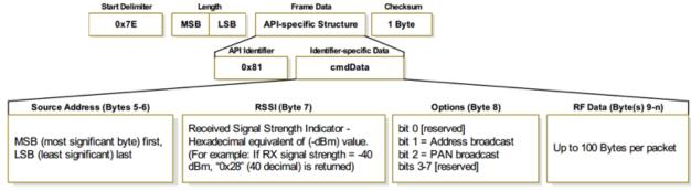
Bytes 5-6 contain the source address. An MI6/SPECTRE should ignore the packet if the source address does not match the address they stored as being the paired device.
