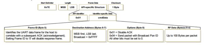
The Frame ID will not be used and must be set to anything except 0x00. The destination address is the XBee address of the desired MI6/SPECTRE to send a packet to. If it is a
